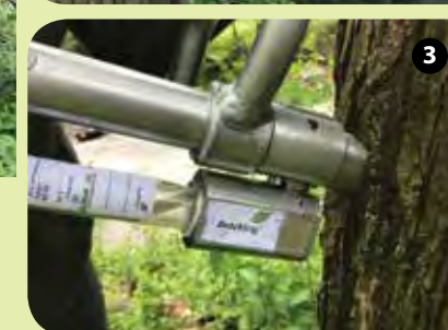
Almstead PHC technician Leo Ibarra (1) and arborist Nick Tripsas (2) receiving training on DutchTrig equipment and treatment. (3) The chisel is designed so that the latest annual ring can be penetrated without penetrating and damaging older annual rings.
