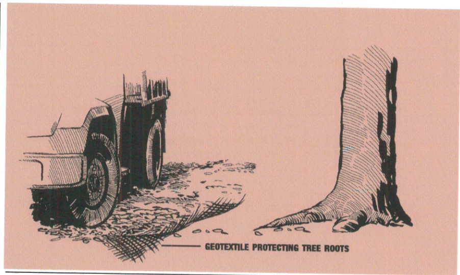
Figure 23. Two to 4 inches of mulch placed on a geotextile sheet protects soils from compaction caused by construction equipment and material storage.
