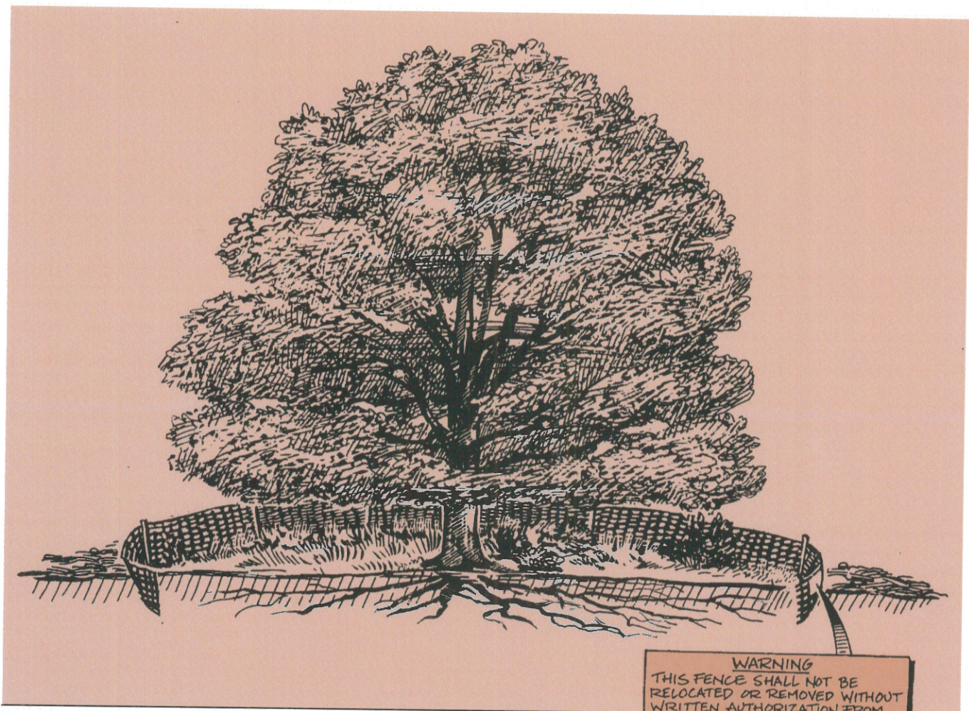
Figure 10. A Tree Protection Zone (TPZ) must be large enough to protect the soil from compaction and the tree from limb and root damage, and it must be explained by a sign.
